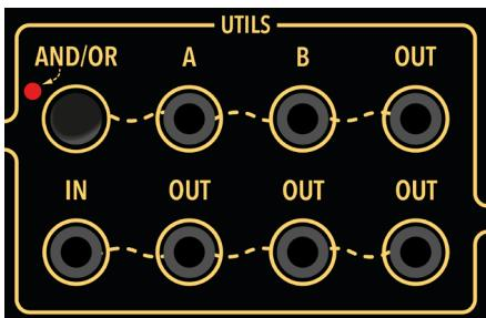
Additionally, it includes a Boolean mixer that allows you to combine 2 input signals, resulting in either an OR or AND operation. To use the AND function, activate the switch (light on).
